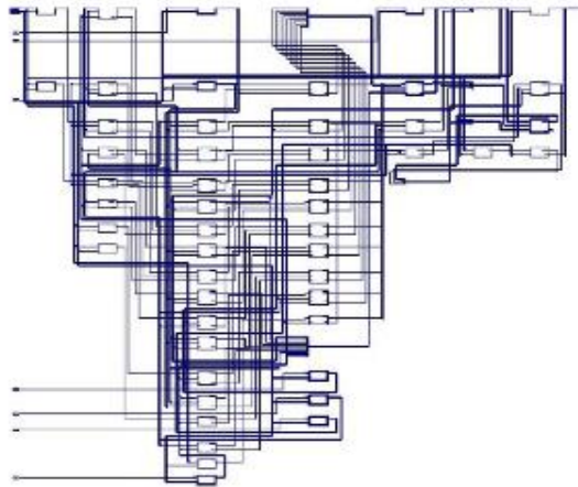
Figure Schematic diagram of Dadda multiplier with modified 5:2 compressors
