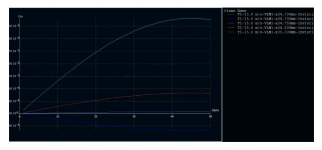
The neutral point was found using XFLR-5 and validated using ANSYS15, the variation of the coefficient of moment v/s alpha. The neutral point was found to be 3.47cm. The validated data from an ANSYS run confirming the location of the neutral point at 3.47cm.Since ansys is a more accurate software and values are obtained by the use of k-w turbulence module and good meshing procedures this value is used for all further calculations.
