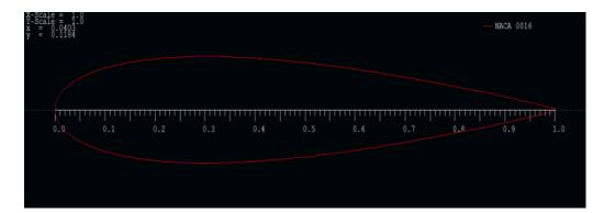
Further, an analysis of the airfoil was done and the neutral point (i.e. where the coefficient of moment is 0) was found to be at 3.47 cm from the tip of the airfoil. Neutral point is basically the point where coefficient of moment is 0 and it coincides with the centre of lift for a symmetric airfoil. Also, the centre of gravity must lie ahead of the neutral point for positive stability. This was since stability was required as explained earlier under stability.
