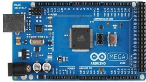
Figure 5: Arduino microcontroller board.
