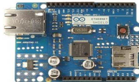
Figure 6: Arduino Ethernet Shield
