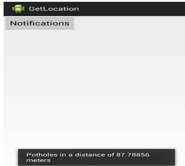
Fig. 7. Pothole alert displayed on the mobile phone.
