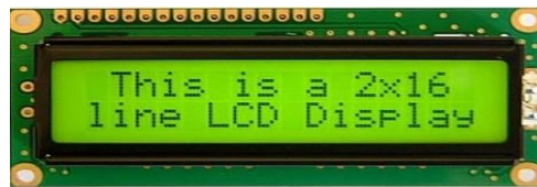
Fig. 2. Liquid Crystal display is to display the load measured in weigh bridge using load cell
