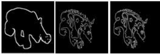
(c) Segmented output after neural network (d) segmented output after prewritten method (e) Segmented output after Roberts method
