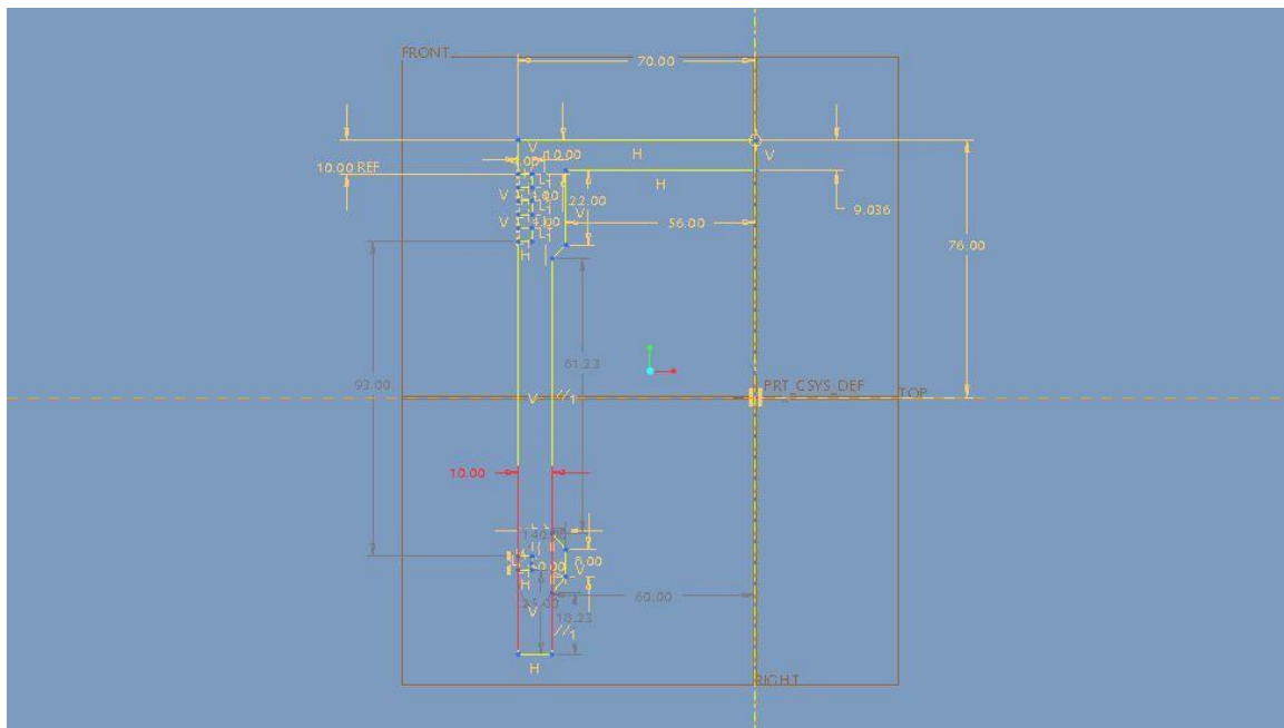
Fig 5.5 Optimized Piston Sketch Pro-E 2d
