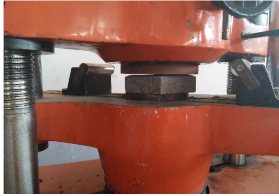
Fig 3.1.1 Before compressive strength of paver block
