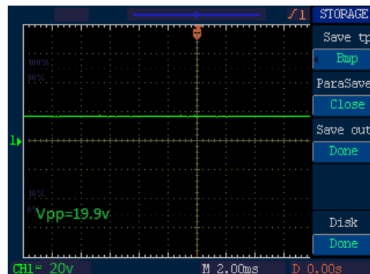
Output DC grid voltage
