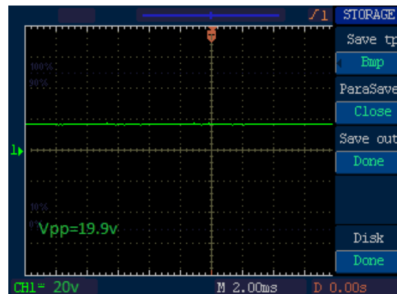
Output DC grid voltage
