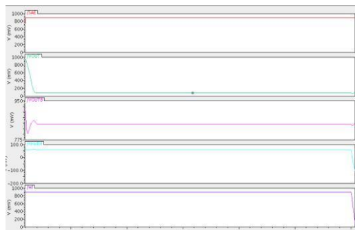
Fig.11 Waveforms Of Read Assist Scheme
