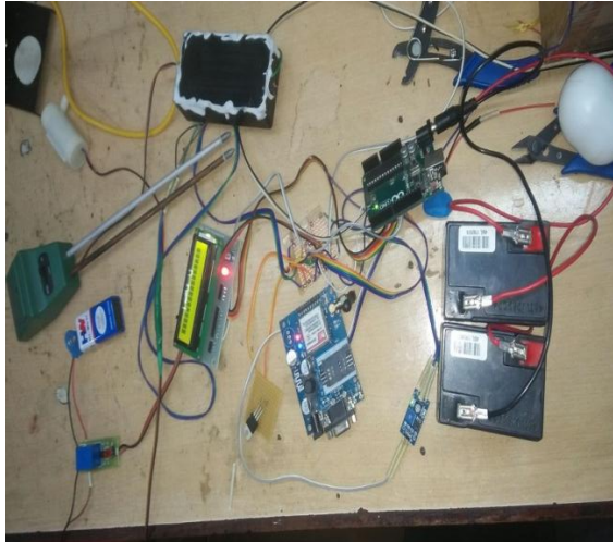
Arduino based Automatic irrigation system
