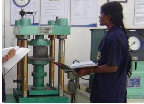
Figure 7: Compressive Strength test
