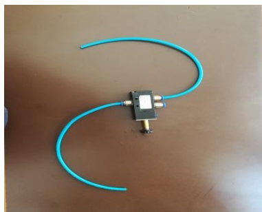
Fig .3 Solenoid valve
