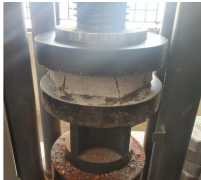
Fig. No.5.1 Compressive strength test
