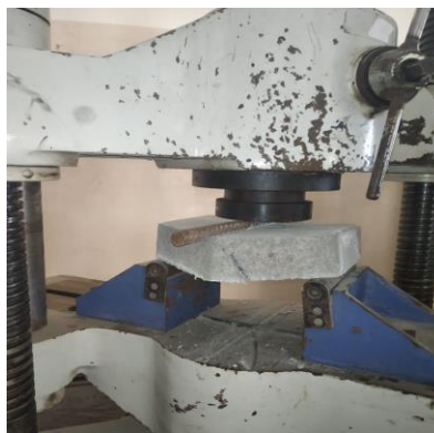
Fig.No.5.2 Flexural strength test
