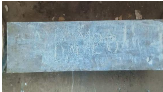
Fig. No.4 Casted beam with curing agent
