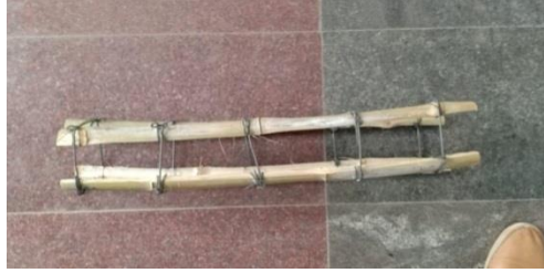
Fig. No.3 Bamboo reinforcement
