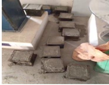
Fig.2 Casting of Moulds
