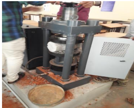
Fig No 6: Testing of cylinder
