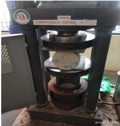
Fig No. 3 Split Tensile Test
