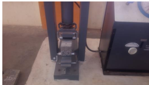
Fig No. 4 Flexural strength test
