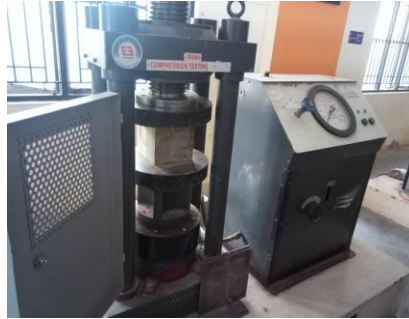
Fig No. 2 Compressive Strength Test
