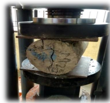
Fig.4 Split tensile strength
