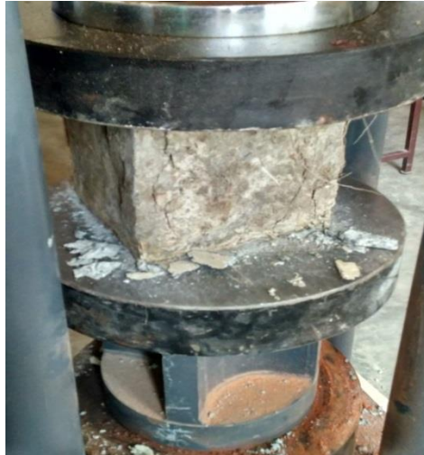
Fig.3 Compression strength test
