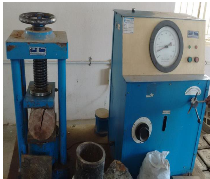
Fig IV. Split tensile strength
