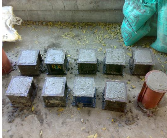
Fig I. Casting of cube specimen
