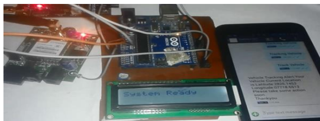
Owner's mobile phone Screenshot of returned SMS to a TRACK VEHICLE request
