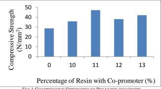
FIG.1 COMPRESSIVE STRENGTH OF POLYMER CONCRETE
