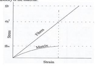
**Fig. 1**: High fibre content in a composite material
