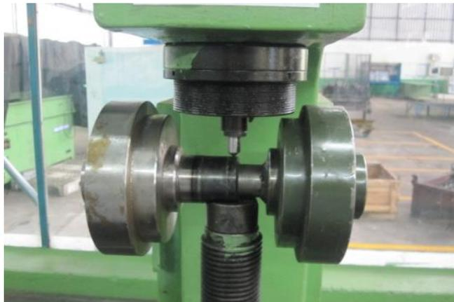
**Assembly kept on hardness testing machine**
