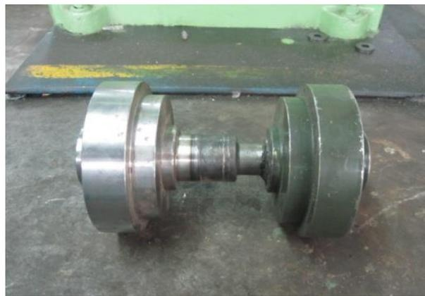
**Counter balance inserted in the flange coupling**
