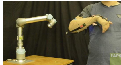
Fig. 5. Test setup with the Universal Robot (left) and the user with the presented sensor sleeve (right).
