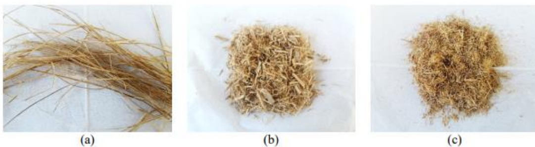
Figure 1. Three types of bamboo fibers: (a) long fibers, (b) short fibers, and (c) powders.
