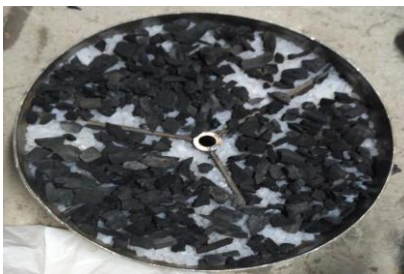
Fig. 5 Inner partition of Desiccant wheel
