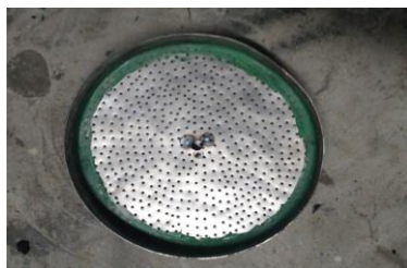
Fig. 5 Inner partition of Desiccant wheel
