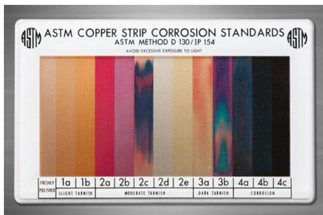
Fig 1. Colour chart for copper strip corrosion test
