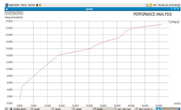
The above graph shows the energy consumption for the number of nodes deployed.
