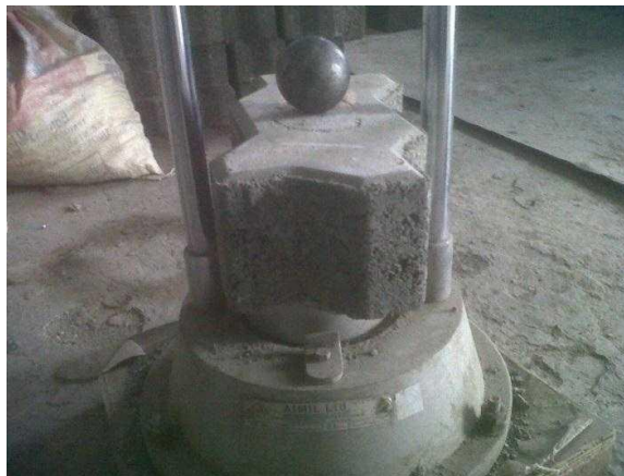
Figure No.2: Impacts testing on paver block using rounded steel ball
