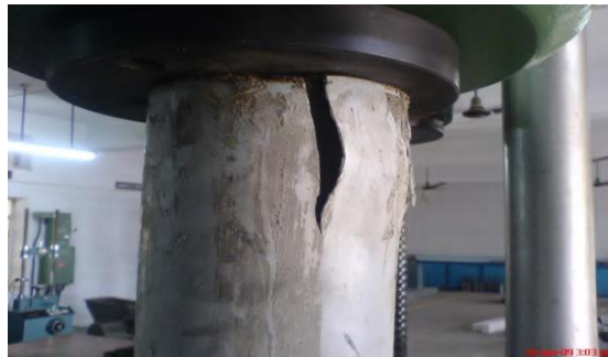
Figure: 5 Failure of PVC confinement
