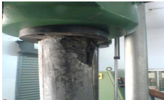
Figure: 3 Failure of ordinary RC column
