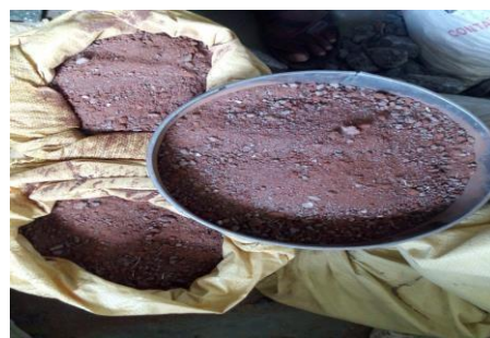
Fig1-Crushed brick masonry wall
