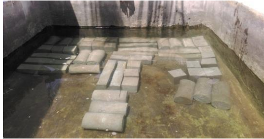
Fig 6-Curing of concrete specimens
