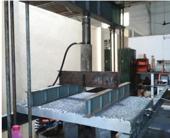
Figure 3 Slab testing setup
