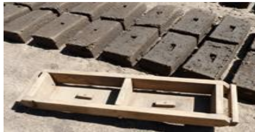
Fig 2.6 Bricks after compaction
