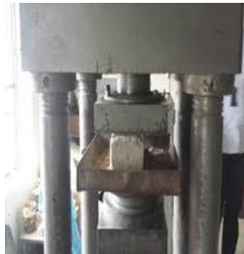
Fig 2.7 Sample before failure
