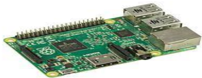
Fig: 6.1 The Raspberry Pi 2B uses a 32-bit 900 MHz quad-core ARM Cortex-A7 processor.
