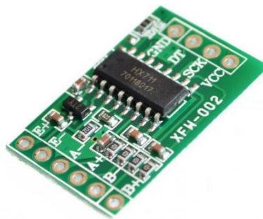
Fig.4.Load cell HX711 IC driver
