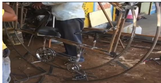
Fig.5 Fabrication of Monowheel
