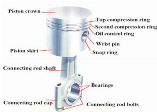
Fig.2: The Piston and its main parts
