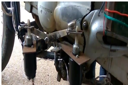
Fig 4. Arrangement of electromagnetic gear changing system.
