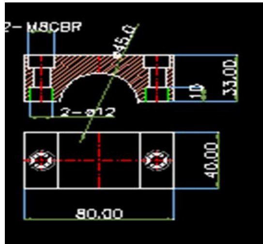
Fig. 4 Drafting of locator top view
