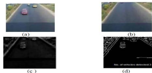
Fig. 3: (a) Real-time image (b) Background image (c) Subtracted image (d) No. of vehicles = 3
