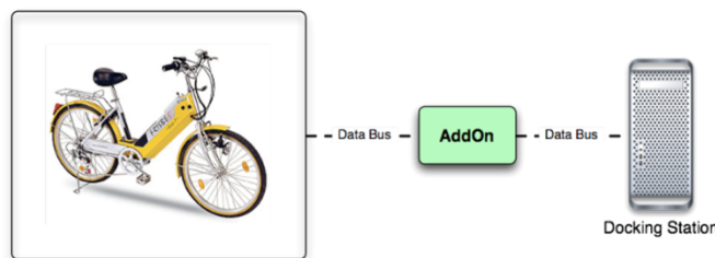
Figure 7 Second option: design of an interface between the vehicle and the docking station.
