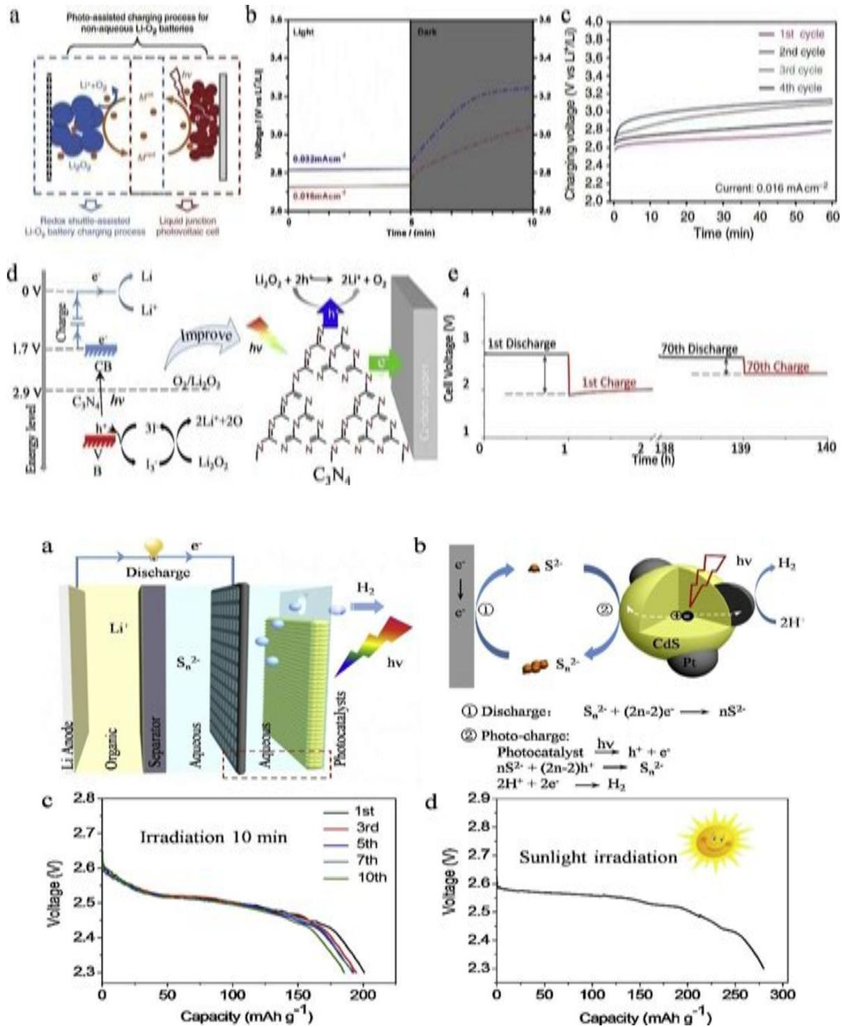
**Fig 7(a)** Schematic of the integration a photo catalyst into a Li-S battery for direct storage of solar energy **(b)** Photo-charge and discharge of solar-powered Li-S batteries. **(c)** The discharge curve saturate of 0.1mAcm<sup>-2</sup> after 10 mini r radiation for ten cycles. **(d)** The discharge curve at a rate of 0.1mAcm<sup>-2</sup> after 2h natural sunlight irradiation.
