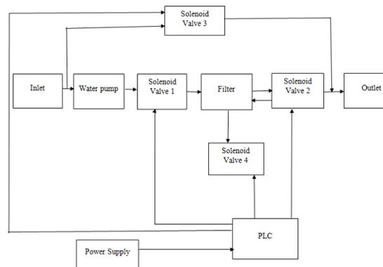
Figure 3.1 Block diagram
