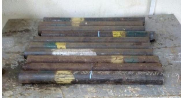
**Fig.2 T91Grade steel tubes.**
