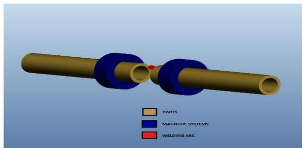
Fig. 1 MIAB Welding Process
