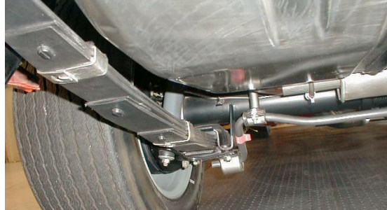
Fig.1 Traditional leaf spring arrangement
