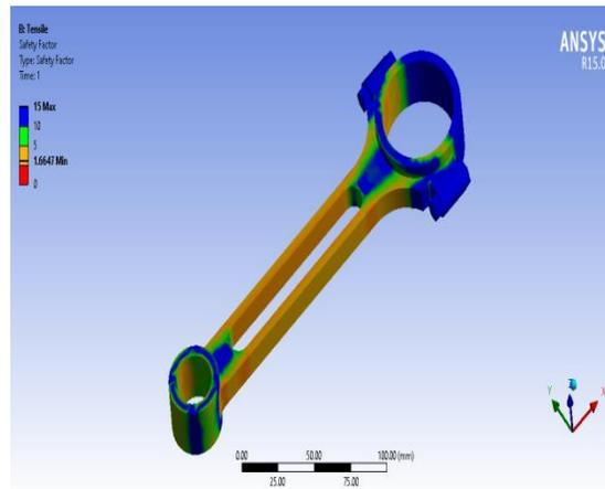
**Fig. 5 (b) Tensile Safety Factor**
