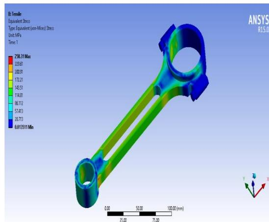
**Fig. 4 (b) Tensile Stress**
