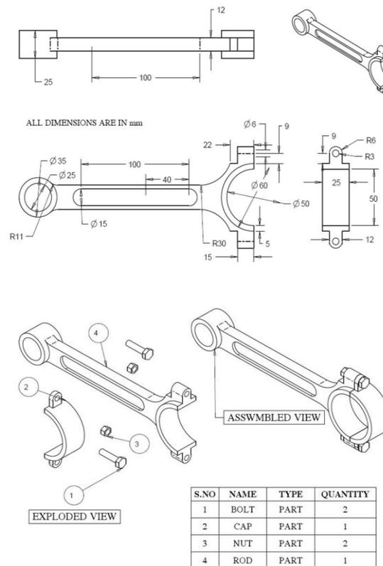
**Fig. 2 Connecting Rod Model with Dimension**
