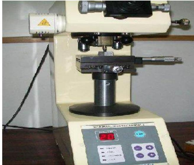
**Figure 1 Vickers micro hardness tester**
