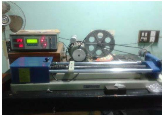
**Figure 3 Digital tensometer setup**
