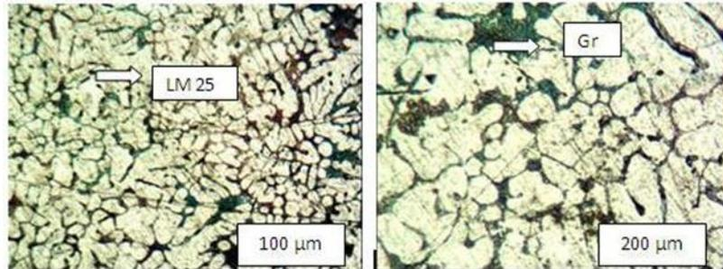
**Figure 4 Optical microstructure of the aluminium alloy LM25 and reinforcement of 5% graphite and 5% of boron carbide with (a) 100×, (b) 200×**
