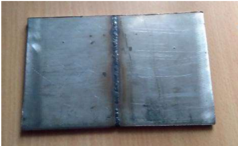
Fig 2. TIG Welding Work piece
